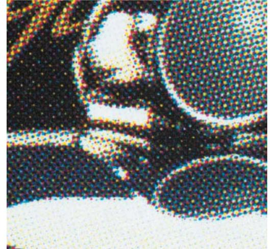
Using stochastic screens gives greater detail. Here, the same image has been printed using two different screens, Heidelberg Diamond Screening (FM), below and Heidelberg I.S. (AM), above. The image has been printed by Billes Tryckeri in Sweden and the detail has been scanned at 1000 percent. (Please note that these are low res pictures and will not do the screening justice if printed out)
