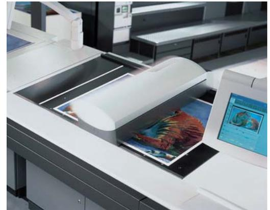
*This Prinect Image Control option from Heidelberg is essentially a spectrophotometer for controlling colour on press.*
