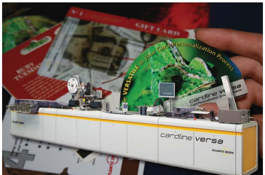
The Cardline Versa from Atlantic Zeiser can produce up to 50,000 cards of various materials per hour.
