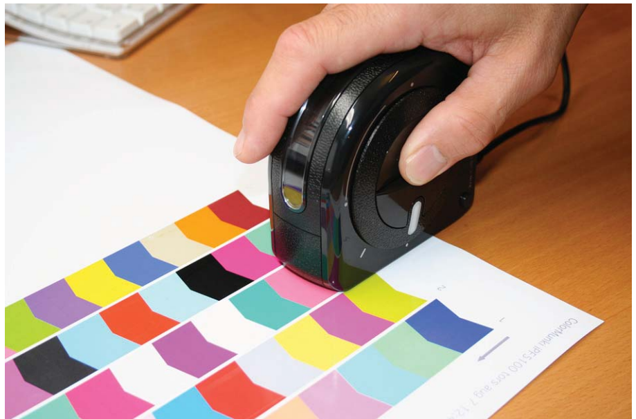
The testforms for Color Munki use a smaller number of larger-than-normal colour patches in order for the user to be able to measure them in a sweeping 'freehand' movement.
