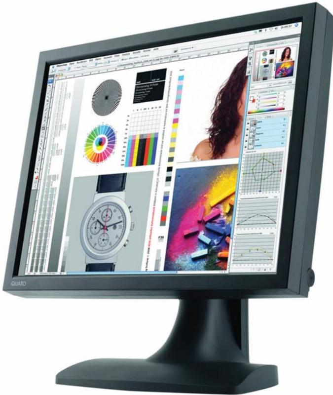
*The Quato monitor Proof View 700 is a high end LCD-monitor with a brightness of 700 cd/m<sup>2</sup>, and a colour gamut large enough for accurate softproofing of both gravure printing and quality offset on coated papers.*
